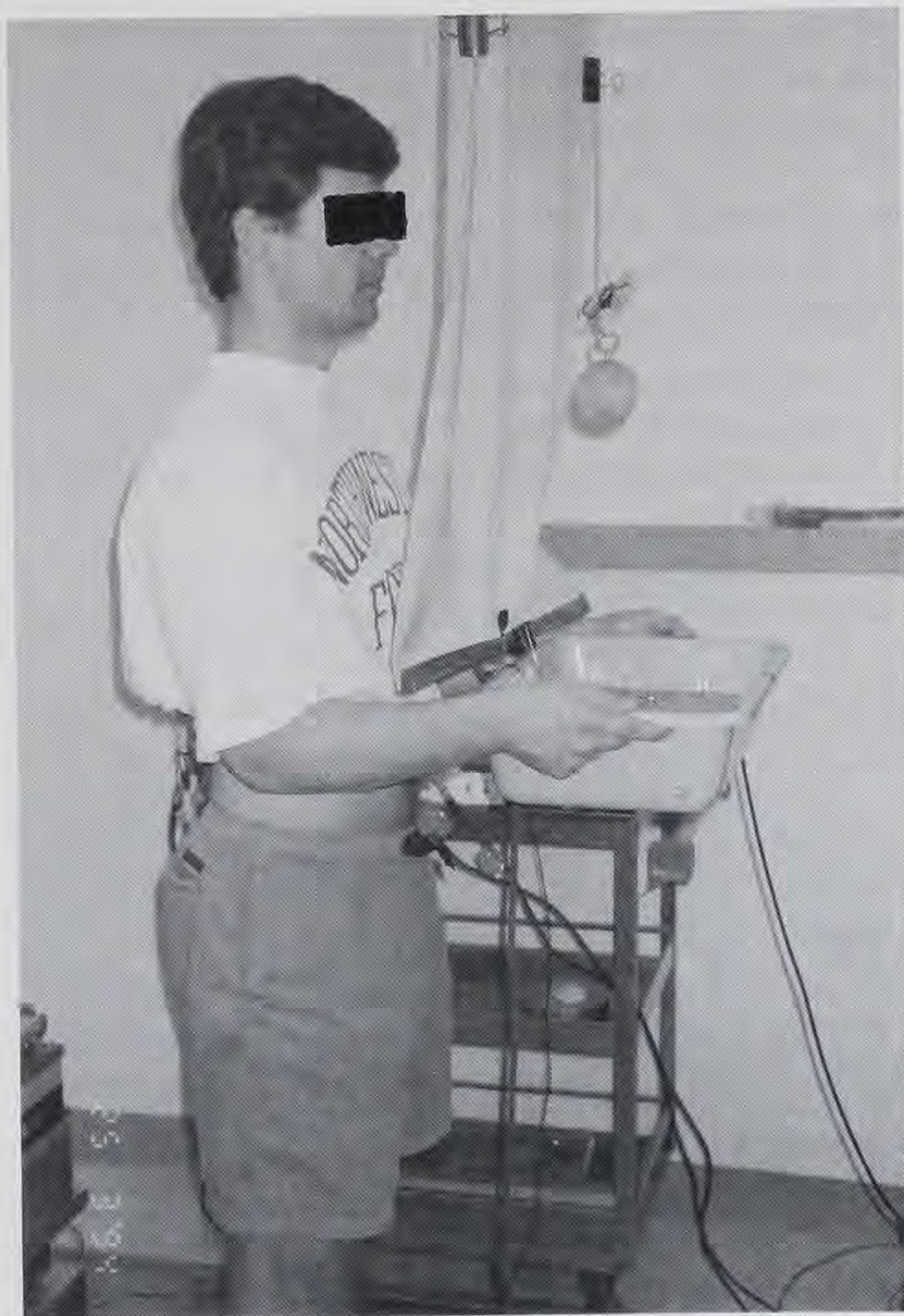
Figure 1. The set-up for the sudden applied load as used in the vibration study (Study 1). A weighted tennis ball was dropped onto a pan, equipped with microswitches for indicating the instant when the ball hit the pan.
