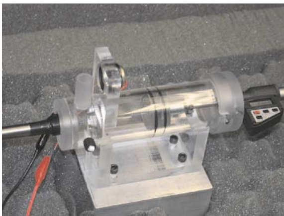
FIGURE 4. Photograph of the prototype acoustic plethysmograph.
