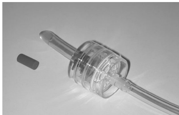
Fig. 1 Microvacuum sampler for use with ASTM Practice D7144.
