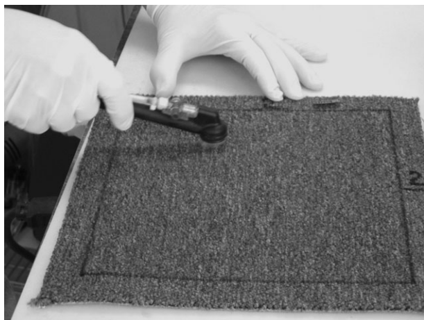
Fig. 5 Microvacuum wet sampling method.
