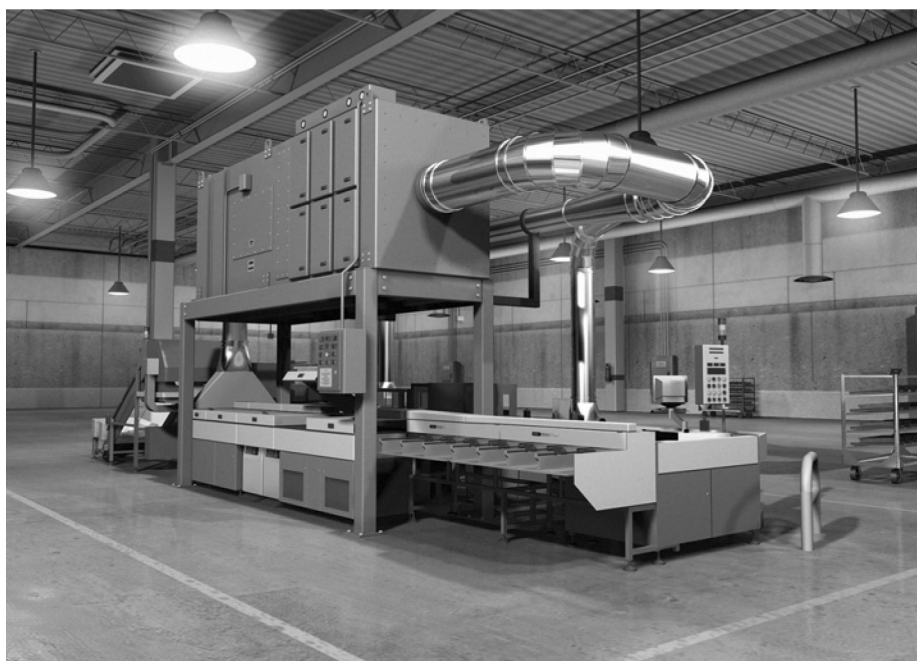
FIGURE 6. Ventilation and filtration system installed on a USPS Advanced Facer Cancellor System (AFCS). The filter/fan housing suspended above the AFCS has a total airflow of 8000 cfm ( 3.8 \text{ m}^3/\text{sec} ).
