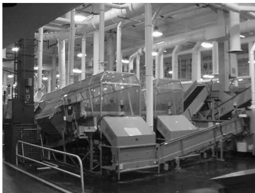
FIGURE 2. Part of the ventilation and filtration system installed on a USPS 010 Culling System. Note the numerous small ducts leading from individual local exhaust ventilation hoods placed above critical areas of the system. All of the small ducts lead back to one of the 18,000 cfm ( 8.5 \text{ m}^3/\text{sec} ) units tested as part of this study.
