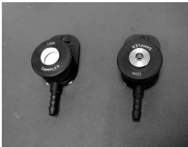
Fig. 2 IOM personal inhalable aerosol 2 \text{ L min}^{-1} sampler (left) and the modified 0.3 \text{ L min}^{-1} version (right).
