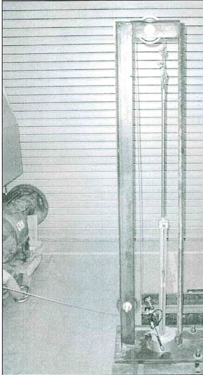
Figure 7 Hydraulic Cylinder and Pulley System for the Pull-to-Failure Test.
