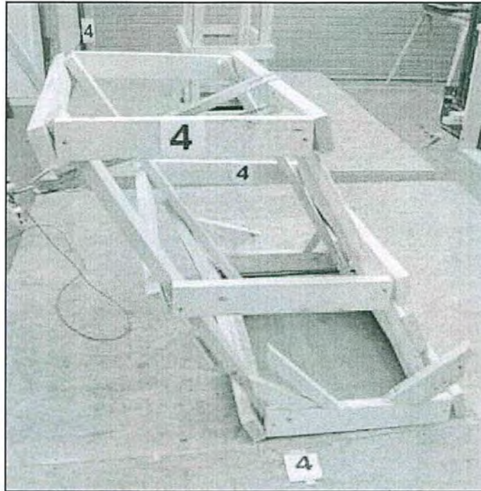
Figure 8. After the PTF test was conducted on a Job-Built system.
