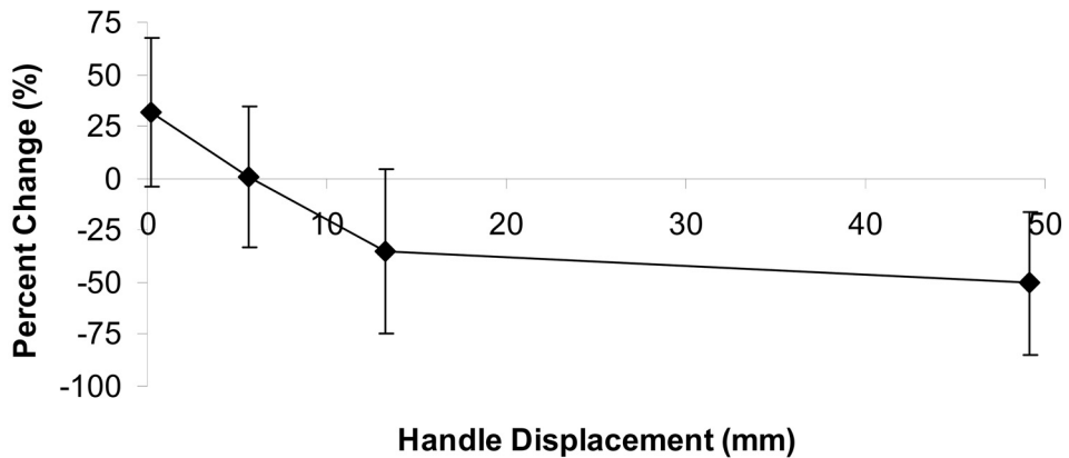
Figure 7. Percent change in stiffness from before tool use to immediately following tool use for predicted handle displacement (mm) (mean and SD).
