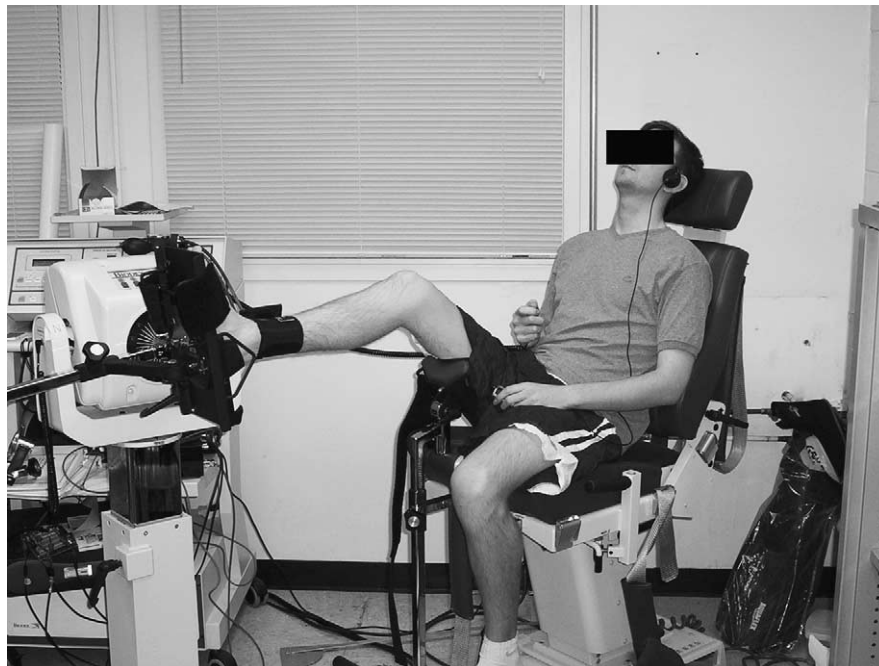
Fig. 1. Subject seated in Biodex System 3 dynamometer for JMS testing.
