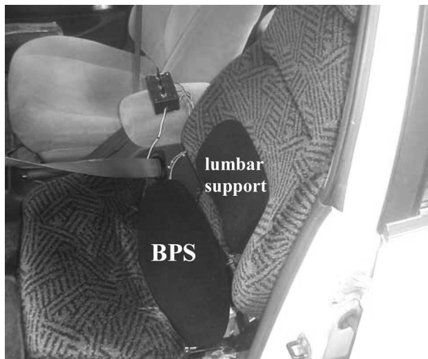
Figure 1. The new seating design as implemented in the testing vehicle. BPS = back part of the seat.
