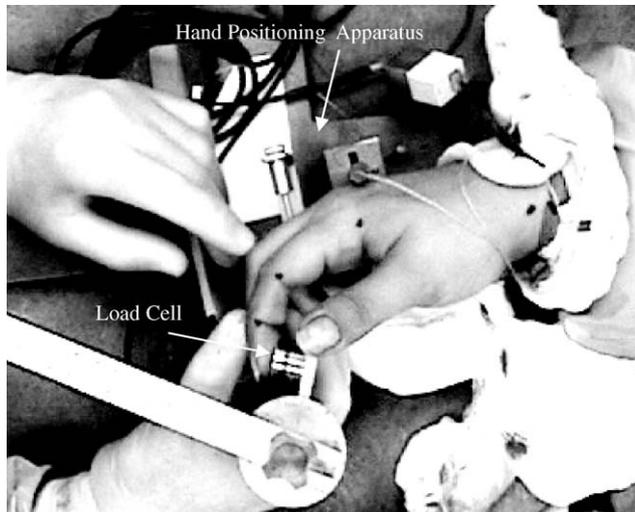
Fig. 1. View of experimental setup from above. The subject's hand is stabilized in a thumb up posture using the hand positioning apparatus and the joint postures are recorded with a video camera. The fingertip force is measured with a six-axis load cell as the FDP and FDS tendon forces are recorded with two buckle force transducers (not visible). Estimated joint centers of rotation are marked.
