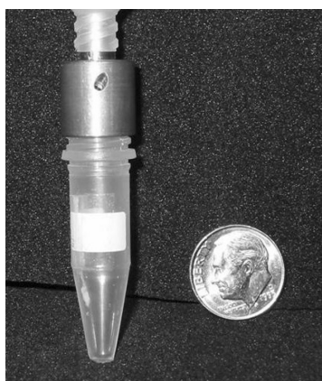
FIGURE 1. Personal cyclone sampler with microcentrifuge tube (MCT) (18-mm coin shown to indicate scale)
