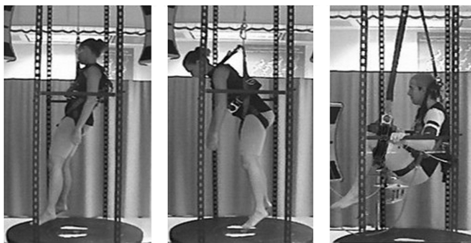
FIGURE 1. Typical postures for the CHEST, BACK, and ACCESS suspension tests. Mean back angle (from vertical) for the BACK suspension was 41°.
