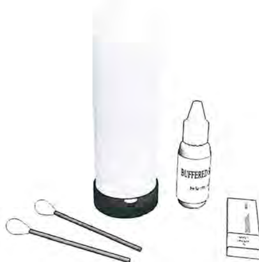
Figure 2. Handheld assays are antibody-based tests that are often employed in the field to give presumptive information about a sample.
