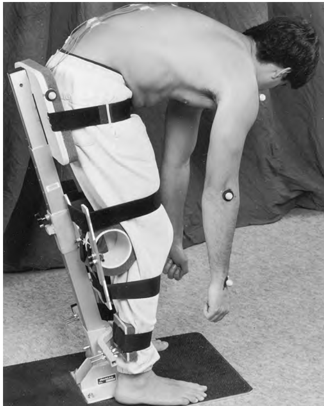
Figure 1. Subject at a fully flexed posture in the restraint stand, secured by thigh and calf straps.
