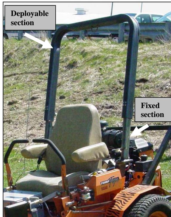
**Figure 6. AutoROPS on a Scag Commercial Mower**
