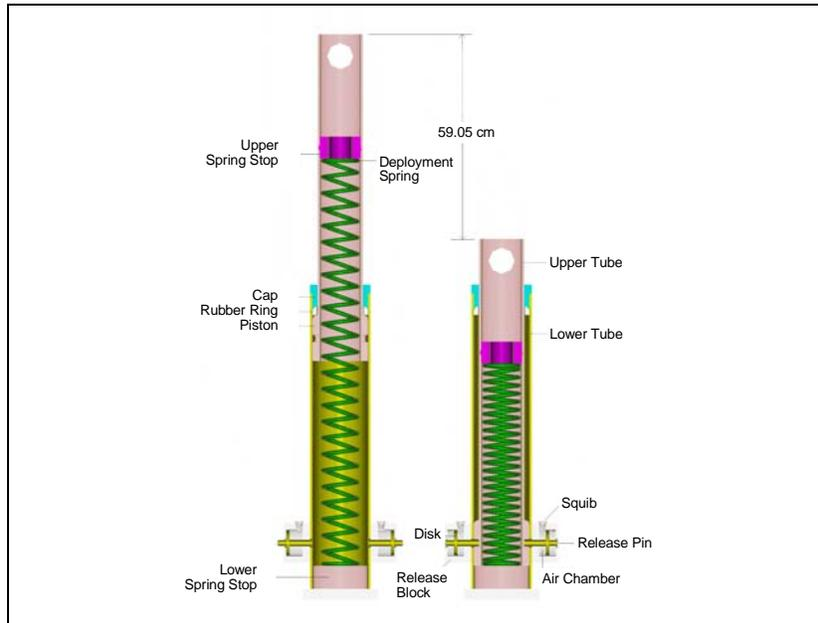
**Figure 3. NIOSH First Generation AutoROPS in Deployed Position and Retracted Position**
