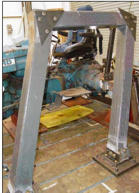
**Figure 9 Composite ROPS after Static Testing**
