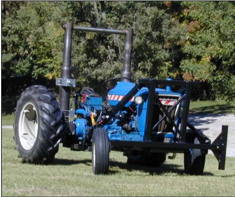
**Figure 2. Ford 4600 after Remote Control with First Generation AutoROPS - 1999**
