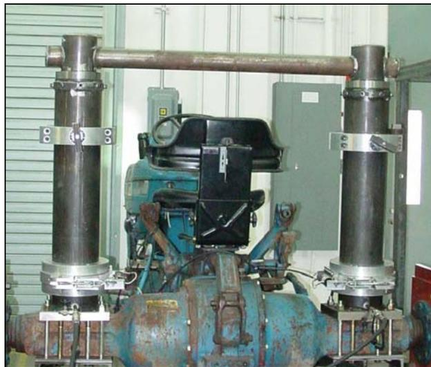
**Figure 4. Second Generation AutoROPS on Ford 4600 in Lab**
