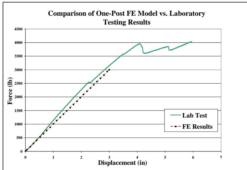
**Figure 7. Composite Lab and FE Comparison**
