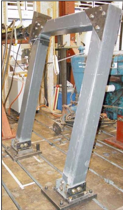
**Figure 8 Composite ROPS before Static Testing**
