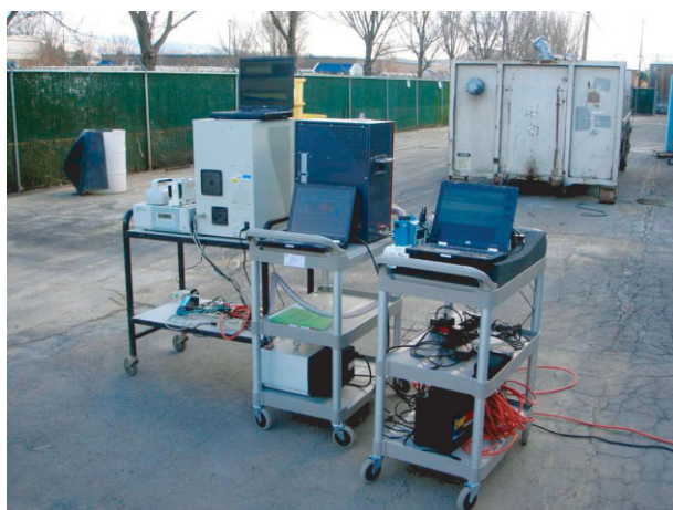
FIGURE 2 | Example of field application of instruments needed for real-time measurement of number, mass, size distribution, and surface area.
