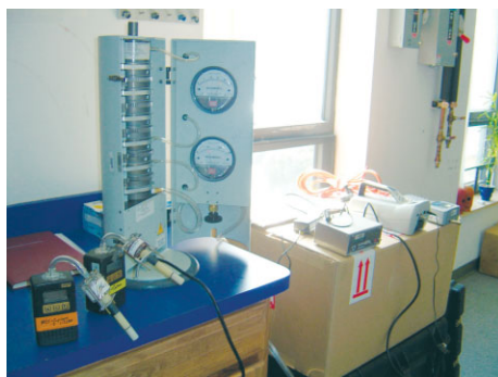
FIGURE 3 | Examples of different sampling instruments used to measure occupational exposure to nanoparticles including the determination of real-time particle number concentrations and size-fractionated mass concentrations.
