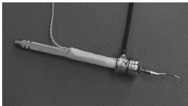
Fig. 2. Modified periodontal scaling tool. The pressure sensor is located under the thin latex sleeve and the six-axis load cell is between the handle and the tip. The cables were of sufficient length to not interfere with scaling.
