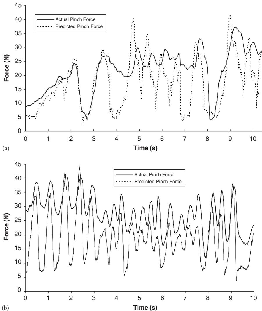
Fig. 6. Predicted and actual pinch force–time series from a scaling task for an experienced (a) and an inexperienced (b) dentist. The predicted force is based on the tip forces and the model. Although there is some error in the middle portion of the sample, the model gives a reasonable approximation of the maximum and minimum pinch forces during the task for the experienced dentists, but has difficulty tracking the force changes for the inexperienced dentist.
