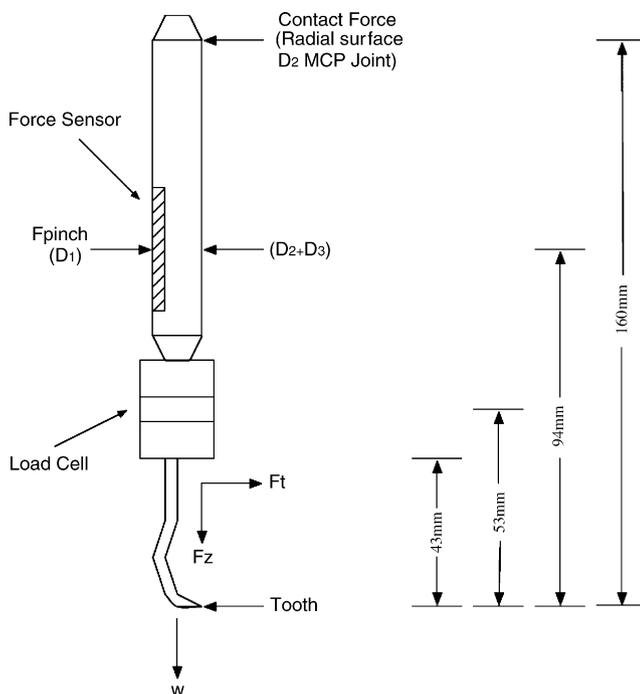
Fig. 3. Periodontal scaling tool free-body diagram with the six-axis load cell and all applicable forces. Dimensions are to scale. The forces  $D_1$ ,  $D_2$  and  $D_3$  (thumb, first and second digit, respectively) denote the location where the user applies the pinch grip. The contact force at the MCP joint is where the end of the tool rests against the user's hand.
