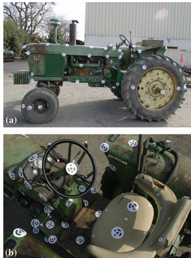
Figure 1. Images used in digital tractor mock-up creation with 'coded targets' around the tractor cab (a) and around the tractor body (b).
