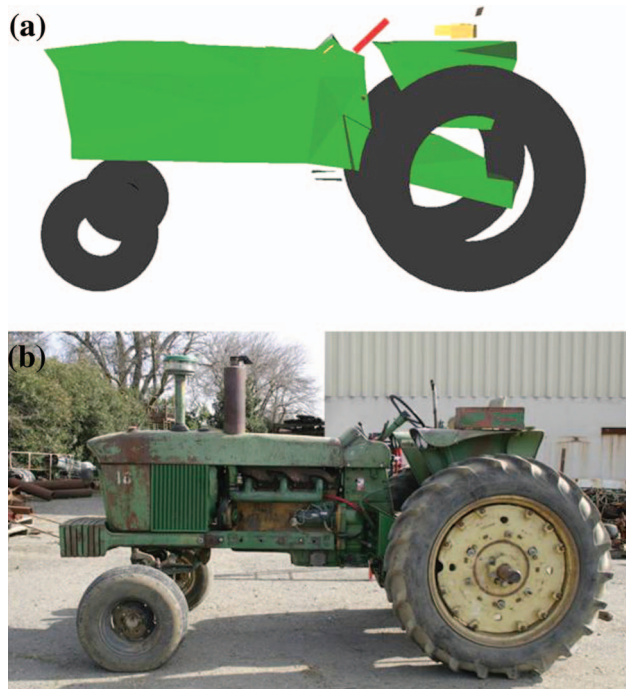
Figure 2. Example of a 3-D digital tractor mock-up (a) of a non-roll over protection structures (ROPS) tractor (b).
