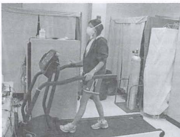
Figure 6. Measurement of physiological parameters of a subject wearing a FFR walking on a treadmill (with permission from NIOSH).
