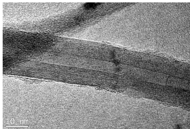
Fig. 1. High resolution transmission electron micrograph of MWCNT. A representative high resolution transmission electron micrograph of the MWCNT shows the distinctive crystalline structure of MWCNT, with this particular MWCNT having 20 walls.
