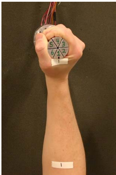
Fig. 2: The orientation of the six measuring arm and the alignment of the hand and arm in the grip force/strength measurement.
