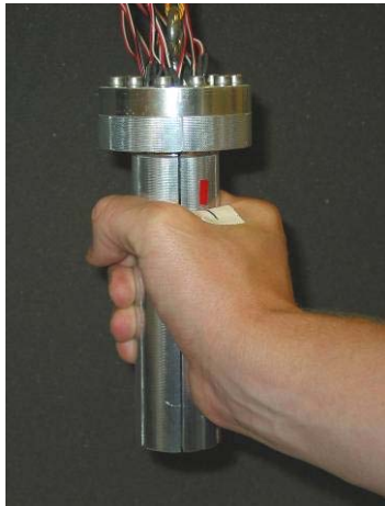
Fig. 1: A 40 mm dynamometer and the hand grip posture used in the grip force/strength measurement.
