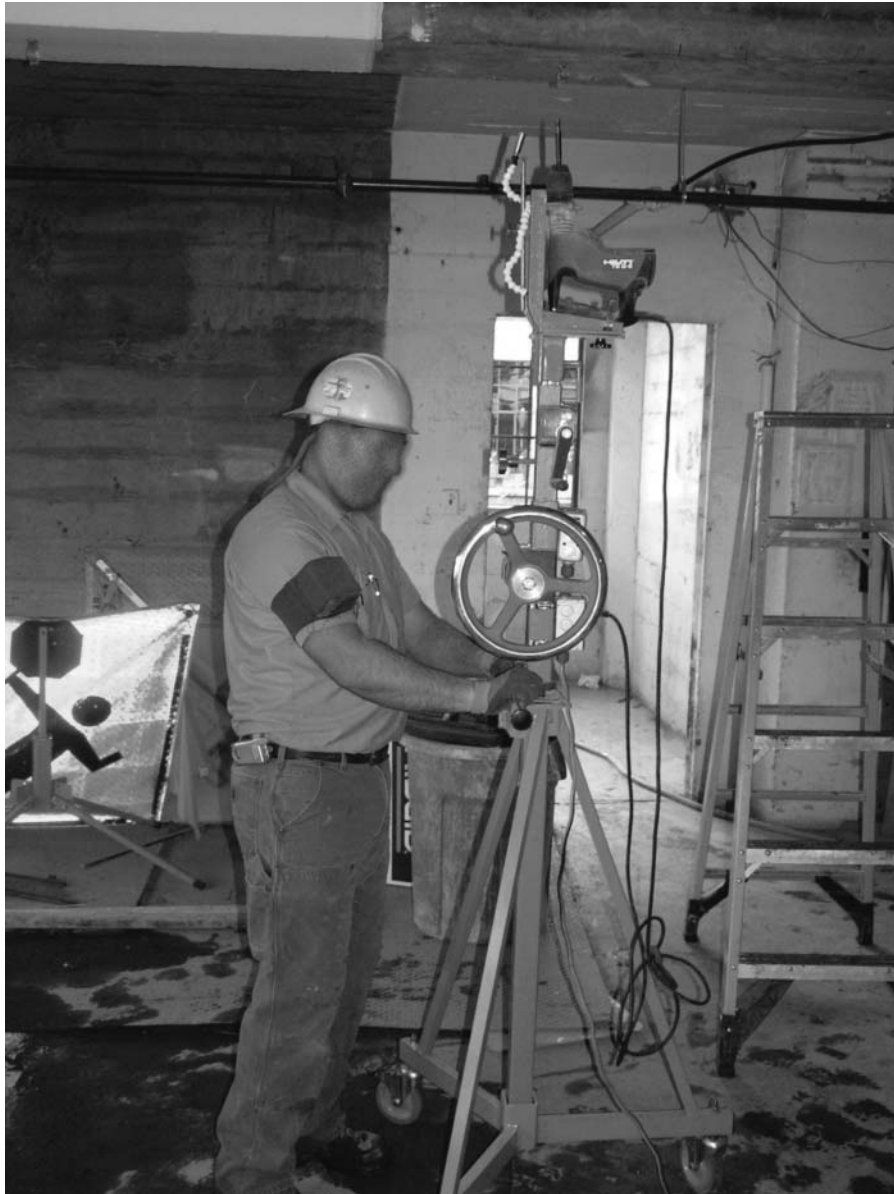
FIGURE 2. New intervention design with wheeled tripod base. Column extends from 2 to 4.7 m. Inclinometer box is attached to upper arm for continuously recording shoulder posture.
