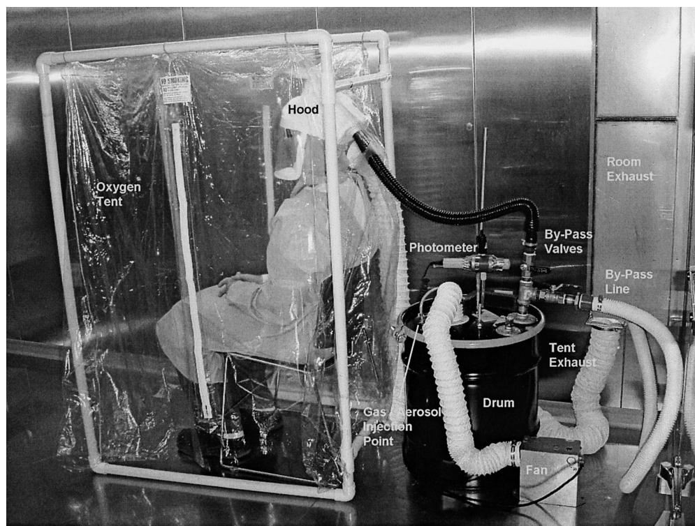
FIGURE 2. Exposure apparatus with subject wearing P APR hood and sitting in an oxygen tent
