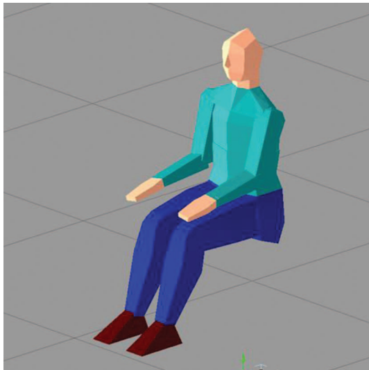
Figure 3. A 3-D virtual human mock-up in a sitting posture created using SAMMIE CAD.
