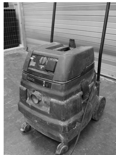
FIGURE 2. Schematic description and photographs of vacuum cleaners that were tested. The Tiger-Vac and the Dustcontrol vacuum cleaners incorporate cyclonic pre-separation upstream of the final filter. The Bosch and Dust Director vacuum cleaners rely upon vacuum cleaner bags to keep debris off the final filters.
