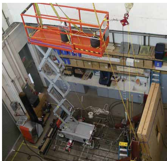
Photo 3 (above): To calculate CG in x and z directions (as shown in Figure 1), four force plates were placed under the wheels of the scissor lift.
