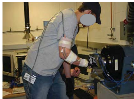
Figure 2.—Measurement of the transmissibility on a 1-D test system.
