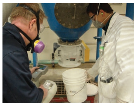
Figure 1 Researchers from the National Institute for Occupational Safety and Health measure the concentration of engineered nanomaterials in the air as a reactor for manufacturing metal oxide nanoparticles is unloaded.
