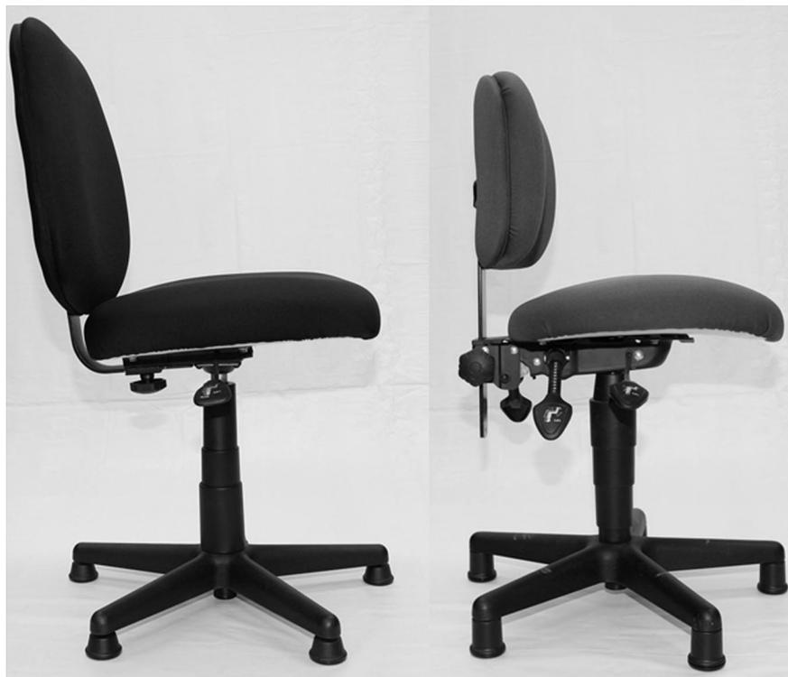
**Fig. 3.** The two intervention chairs. The left chair has a flat seat pan and the right chair has the curved seat pan. The front half of the curved pan slopes forward at approximately 15 degrees. Both task chairs are adjustable in height and swivel. The chairs have no castors so that they do not move during sewing.
