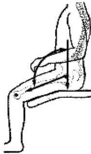
**Fig. 2.** Design of the curved task chair seat pan allowing for a more open thigh-torso angle and preservation of lumbar lordosis.
