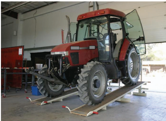
Figure 3. Tractor ramp constructed to capture braking force.
