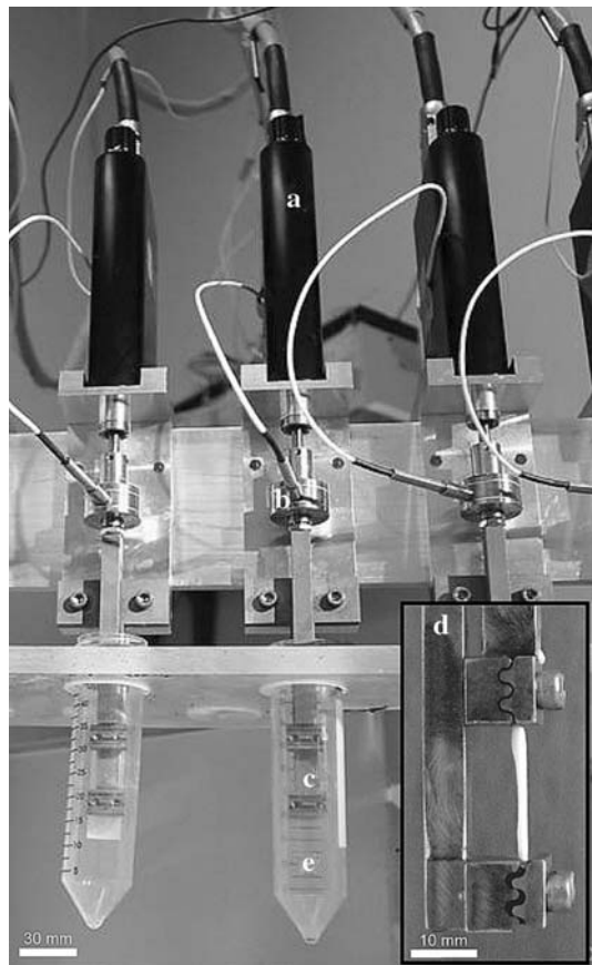
FIGURE 1. Image of three of the six actuators of the loading system. Letters identify system components. (a) Ultra-precision actuator (accuracy \approx 0.75 \mu\text{m} ; speed range: 0.02 \mu\text{m s}^{-1} – 25 \text{ mm s}^{-1} ); (b) load cell (accuracy \approx 0.1 \text{ N} ; force range: \pm 50 \text{ N} ); (c) ridged clamps; (d) close up of a tendon secured within the clamps. Fibrocartilage region can be seen protruding from the upper clamp. (e) Tube which can be filled with saline or media. Water bath not shown.
