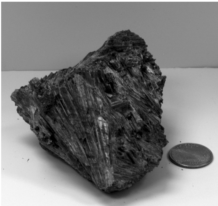
FIGURE 2. Coarsely crystalline (non-asbestiform) actinolite (scale indicated by a 25 \phi piece).
