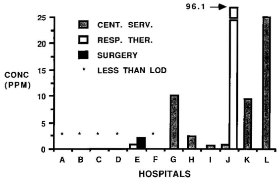
Figure 2. Arithmetic means of the short-term exposure to ethylene oxide (personal samples) in the 12 hospitals. (LOD = limit of detection, CONC = concentration)
