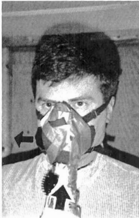
Figure 1. The modified respiratory protective mask used in the experiments. The direction of the air flow is shown.
