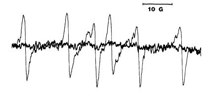
Figure 1. E.P.R. spectrum of free radicals trapped by DMPO in human intestinal content incubations. The spin trap adduct was extracted in ethyl acetate and the spectrum measured under argon at  $25^{\circ}$  C with a Varian E-104A spectrometer. Amplification was the same for both spectra; the higher amplitude trace is from the  $\mathrm{N}_2\mathrm{O}$  incubation, the lower amplitude trace is from the argon control.
