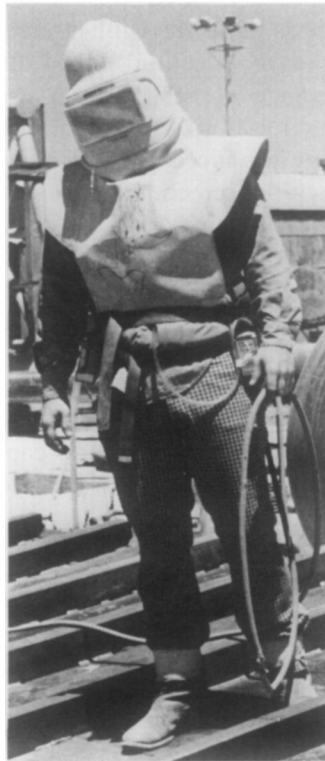
FIG. 2. Sandblaster wearing modern air-supplied hood and pumps for sampling inside and outside hood.
