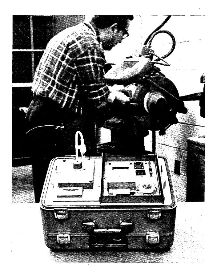
Figure 2. Photo of model RDM-301, recording dust monitor manufactured by GCA Corporation.
