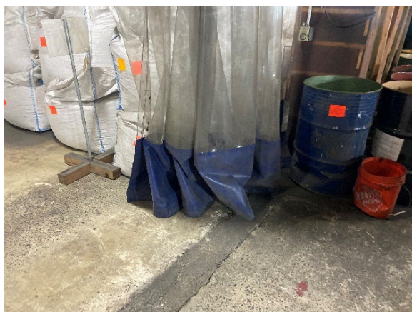
Figure A4. Loose curtain between the main warehouse and the lead melting area, pulled closed while the melting furnaces are powered on. Photo by NIOSH.
