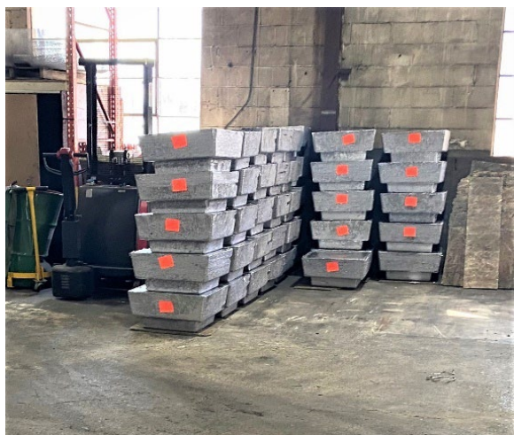
Figure A7. Lead ingots in the warehouse weighing approximately 2,000 pounds each. Photo by NIOSH.
