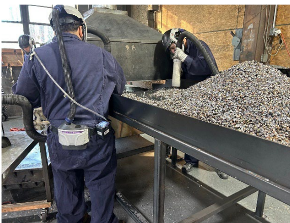
Figure A3. Employees vacuuming rubber from the lead and copper components. Photo by NIOSH.
