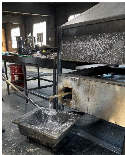
Figure A6. Pouring liquid molten lead into mold. Photo by NIOSH.
