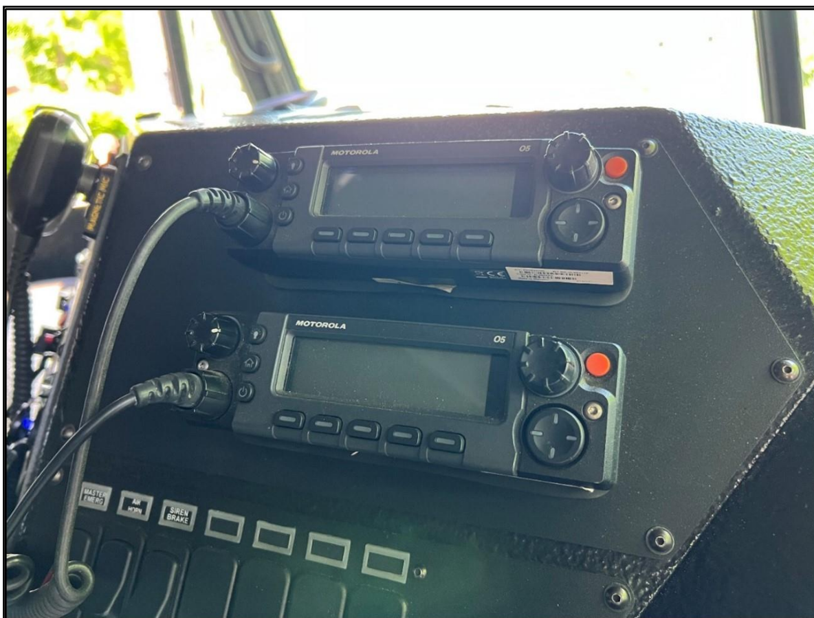
Photo 1. The radio console in the cab of Tanker 17 showing the UHF mobile radio and 700 MHz mobile radio. (NIOSH Photograph)
