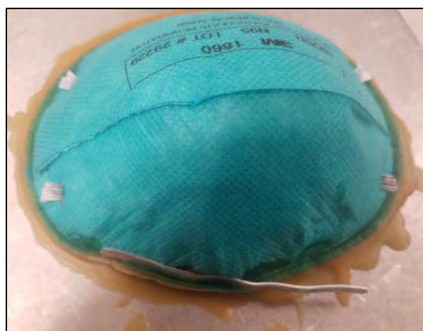
Figure 4: Most amount of product damage observed from Facility Three (the respirator is affixed to a test plate via beeswax).
