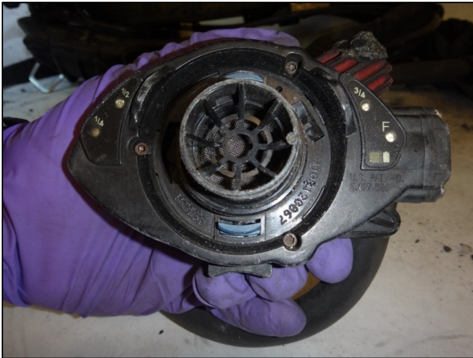
Figure 10: Inside flange, mask mounted regulator
