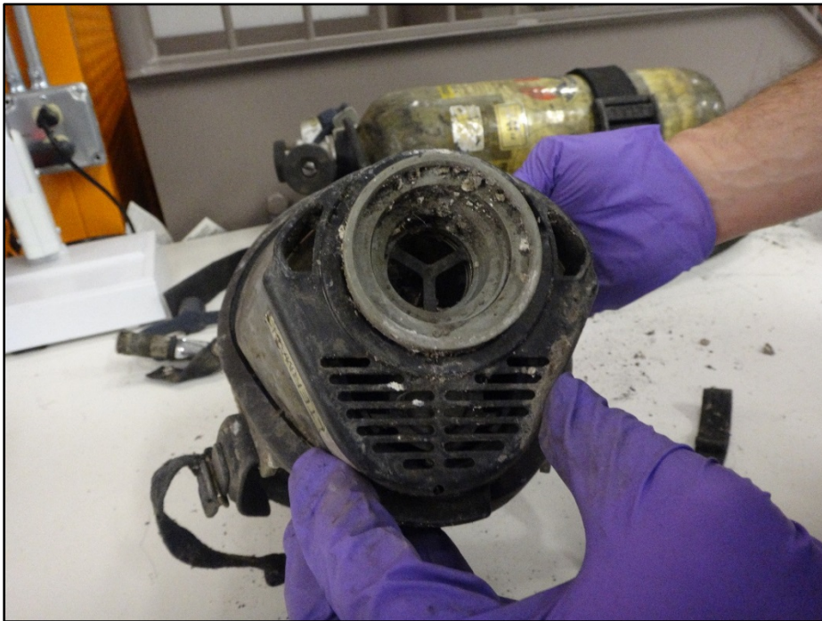
Figure 6: Bottom view of facepiece, debris inside
