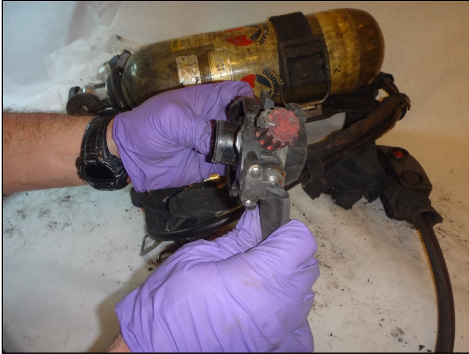
Figure 11: Heat damage to air supply valve
