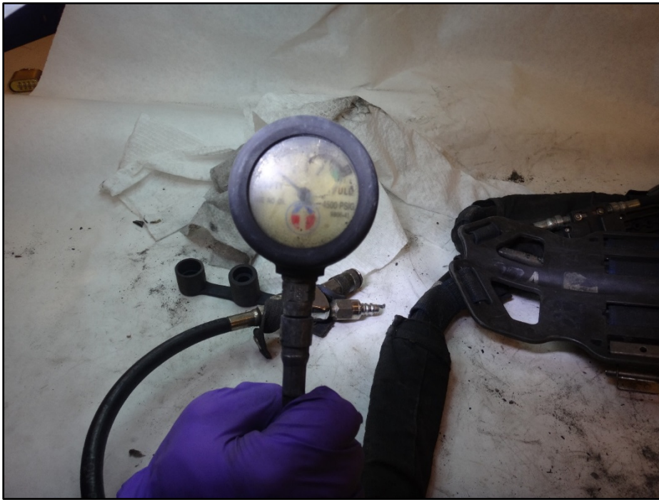
Figure 29: Standalone gauge, lens scratched but readable
