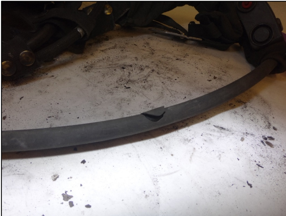
Figure 12: Tear in protective cover of low pressure hose
