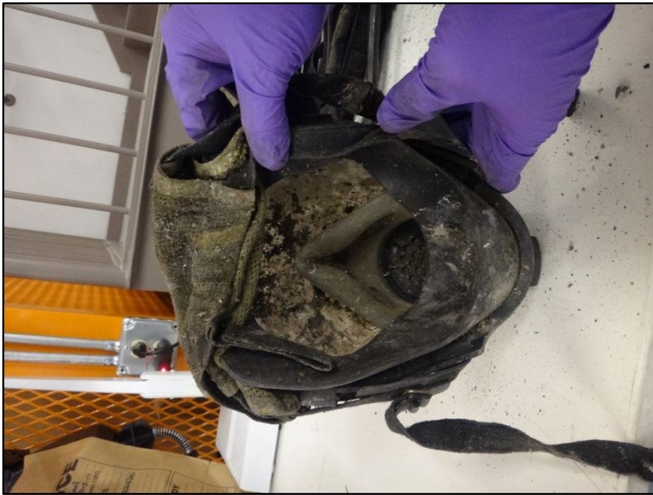
Figure 5: View of inside of facepiece, covered in debris
