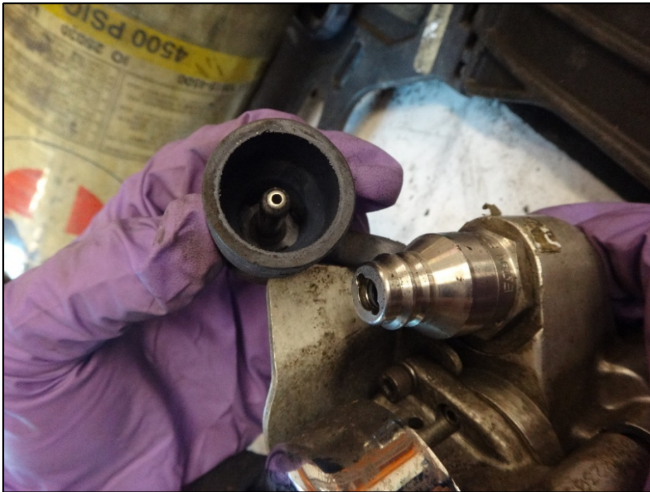
Figure 18: Quick fill port on cylinder attachment
