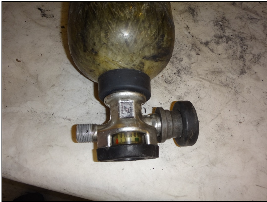
Figure 27: Cylinder threads with readable cylinder gauge
