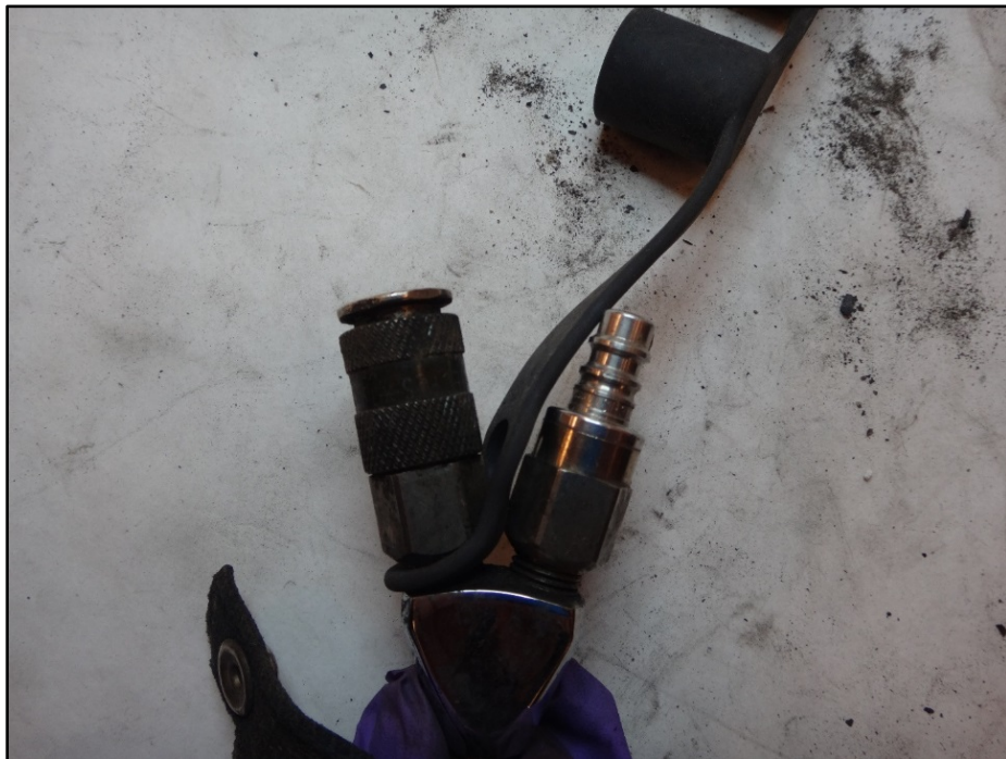
Figure 28: Auxiliary hose, female and male attachments
