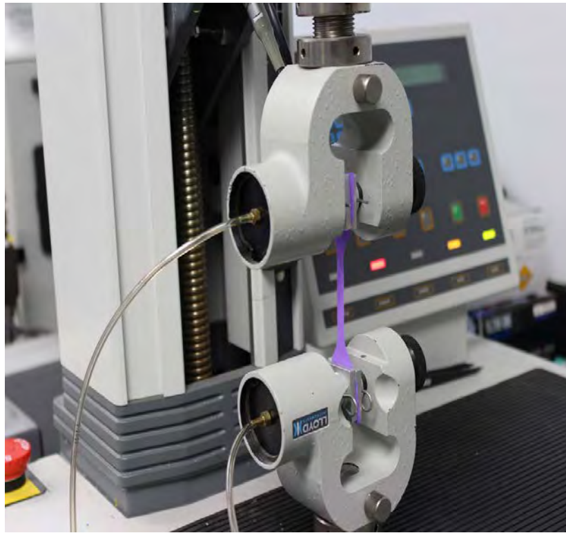
Figure 34. Tensile property testing of glove specimen following application of disinfectant. [Photo credit: NIOSH]
