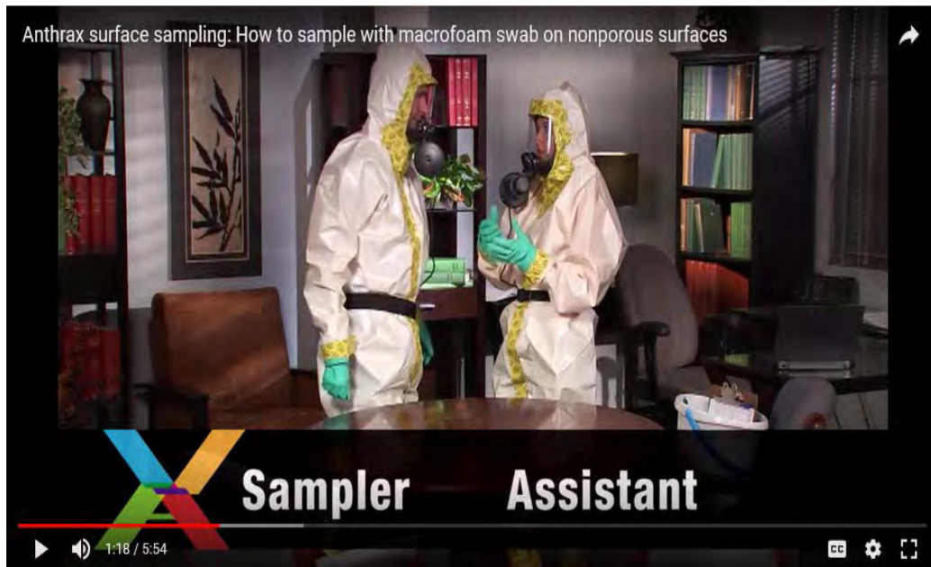
Figure 16. Screen shot of instructional video showing how to sample with macrofoam swab.
