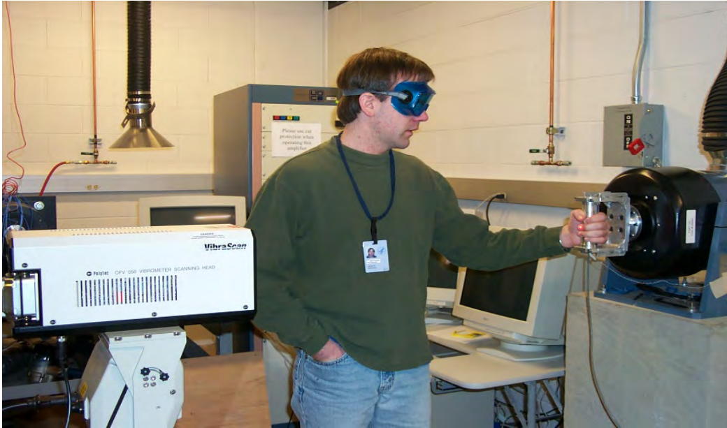
Figure 17. The 1-D hand-arm vibration test system and 1-D scanning laser vibrometer.
