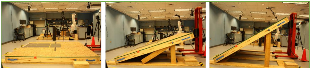
Figure 22. A roofing simulator for the study of roofers' MSDs in the HELD facilities in Morgantown.
