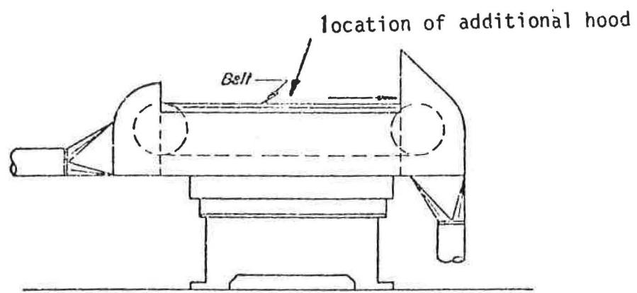
The belt sander having the automatic feeding system was also equipped with a ventilation system, controlling the dust from this feeding system. When the feeding system consisted from a number of narrow belts, small slot hoods were located between each belt. A typical example was a large polisher with a factory-installed ventilation system in one of the furniture shops. In addition, the plant installed a movable hood directly above the polishing area.
