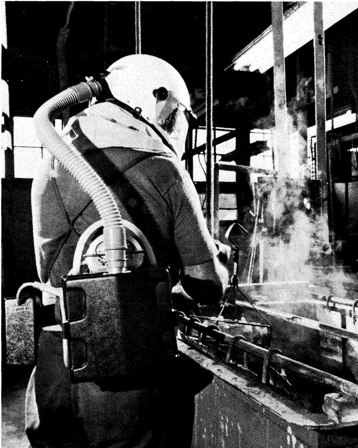
FIGURE 4. - Powered Air-Purifying Respirator (3M Co.).
