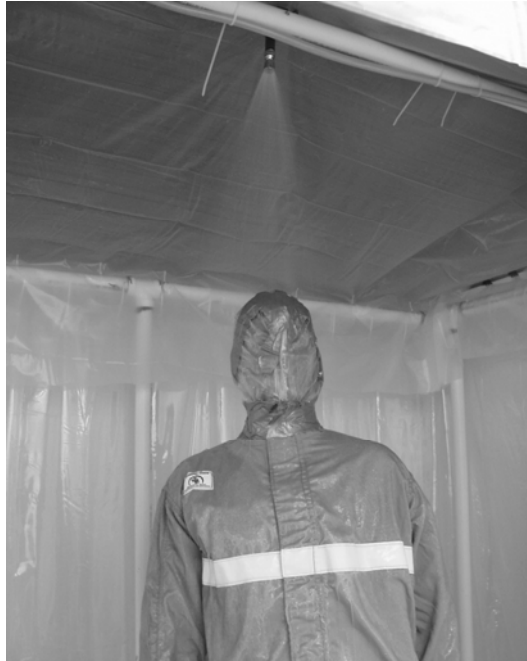
Figure 7 – The “Shower Test” as Applied to a Garment to Measure Liquid-Tight Integrity
