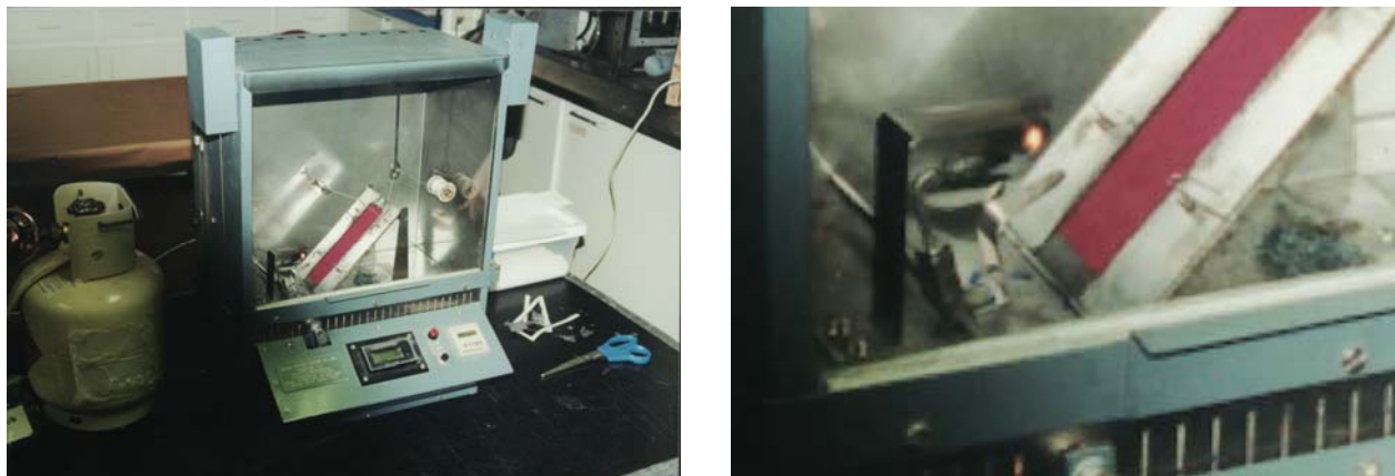
Figure 44 – Fabric Flammability Test Apparatus with Close Up of Flame
