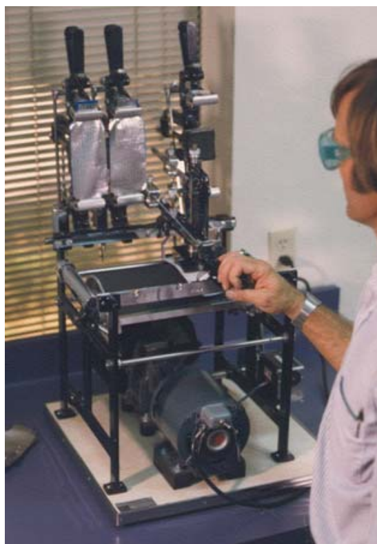
Figure 10 – Wynzenbeek Abrasion Test Apparatus Applied to Protective Clothing
