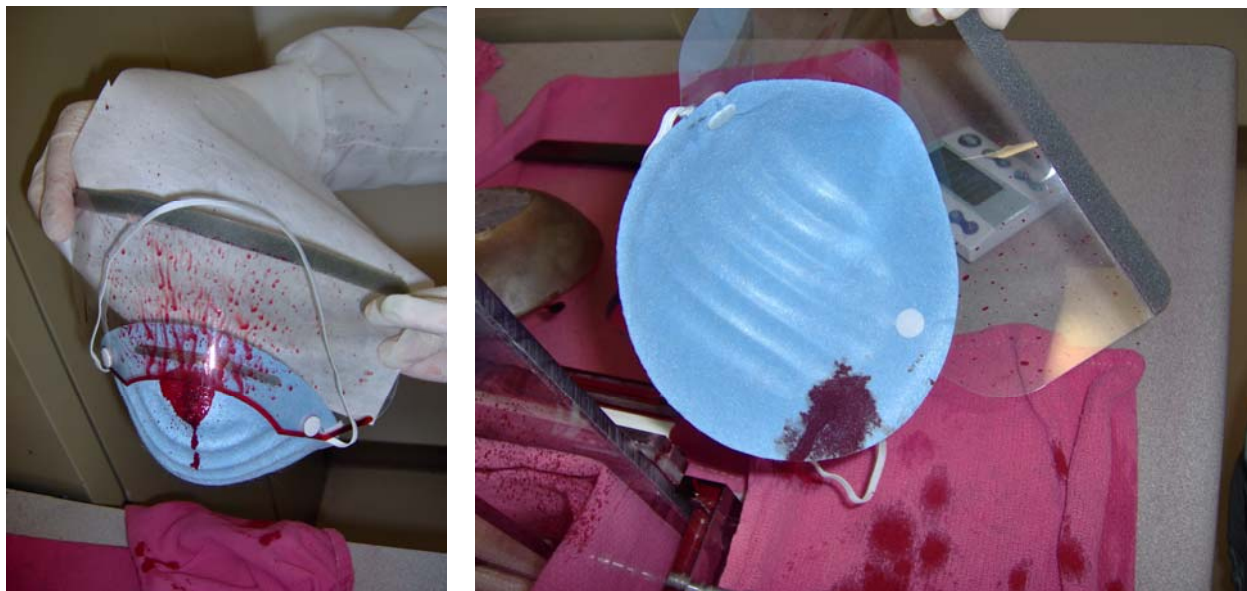
Figure 64 – Two Specified New Target Locations on Medical Face Masks for Liquid Integrity Test
