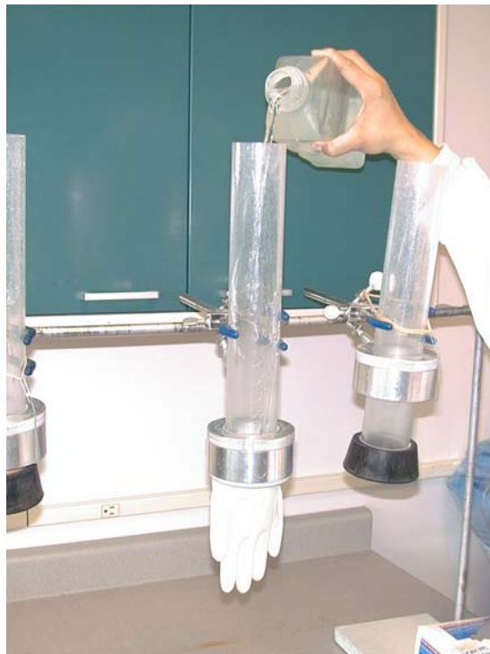
Figure 8 – A Liquid-Tight Integrity Test for Examination Gloves Involving the Suspension of the Glove Filled with Surfactant-Treated Water
