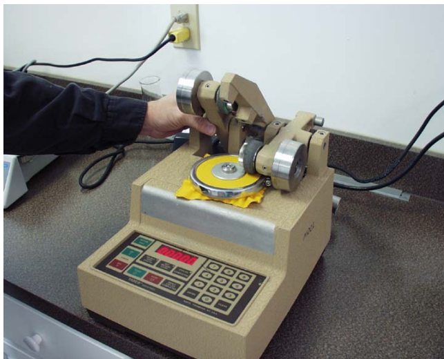
Figure 37 – Taber Abrasion Test Apparatus with Sample Abraded Fabric Specimen
