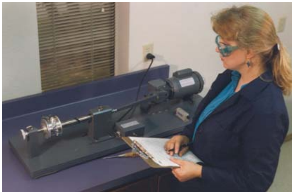
Figure 9 – Gelbo Flexing of Material Specimen Showing Sample in Full Twisted and Compressed Condition
