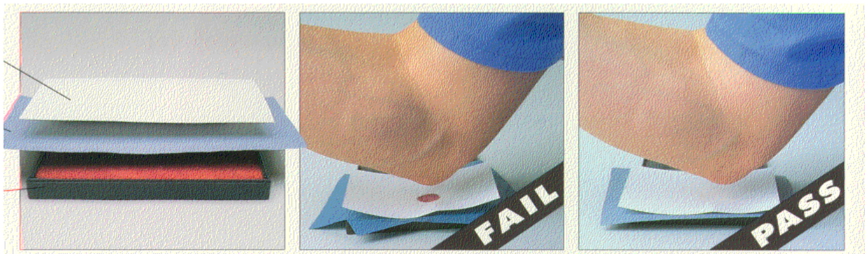
Figure 2 – Elbow Lean Test to Demonstrate Synthetic Blood Strike Through for Protective Clothing Materials
