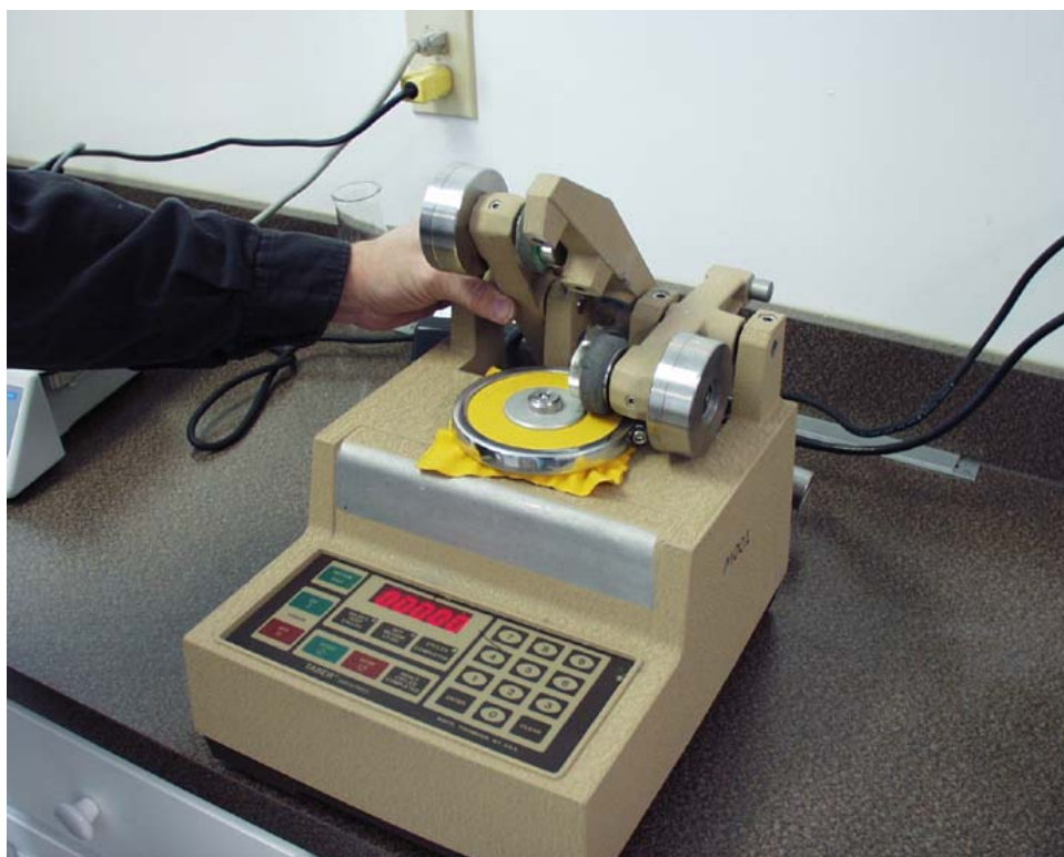
Figure 14 – Taber Abrasion Test Method used for Cleaning Gloves
