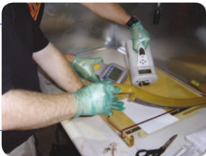
Checking for fiber release during destructive testing of nanofibers deposited on a substrate using optical and condensation particle counters.
