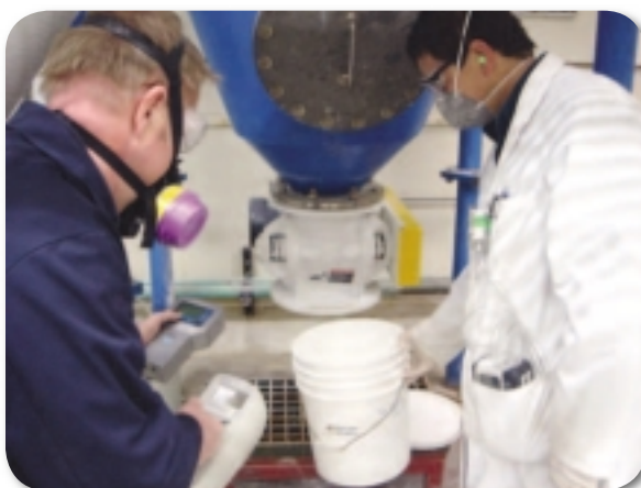
NIOSH monitoring of a worker during a nanomaterial powder production and collection operation.
