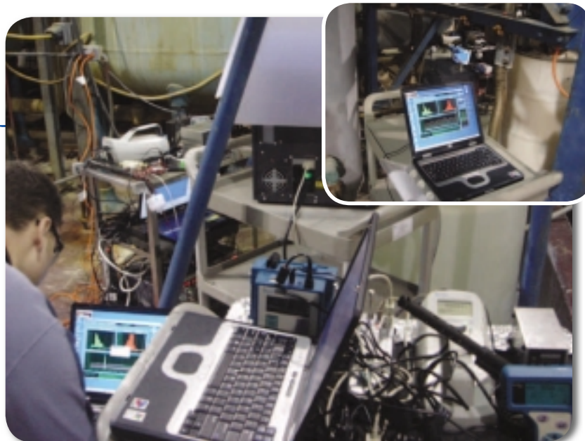
Comprehensive aerosols measurements conducted at different production processes within a primary nanoscale metal oxide production facility. A number of aerosol sampling methods and instruments are used simultaneously to better understand particle characteristics.
