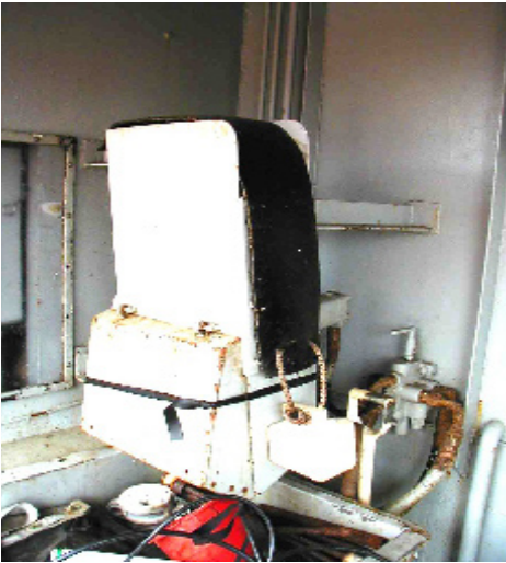
Figure 4: Bait chopper guard made from old conveyor belt material.
