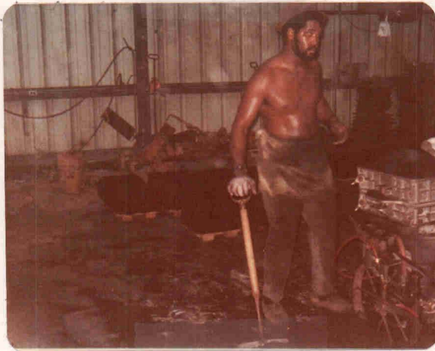
Worker filling casting and mold with basic sand and clay mix.
