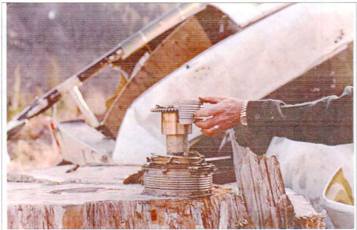
Figure 8. Drive shaft and rear coupling separated.
