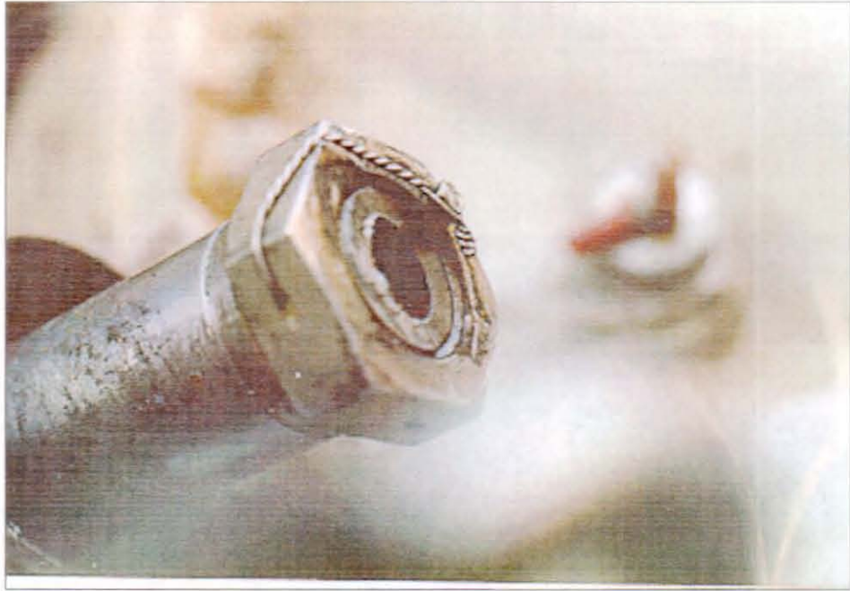
Figure 9. Location of break on right cyclic piston rod.
